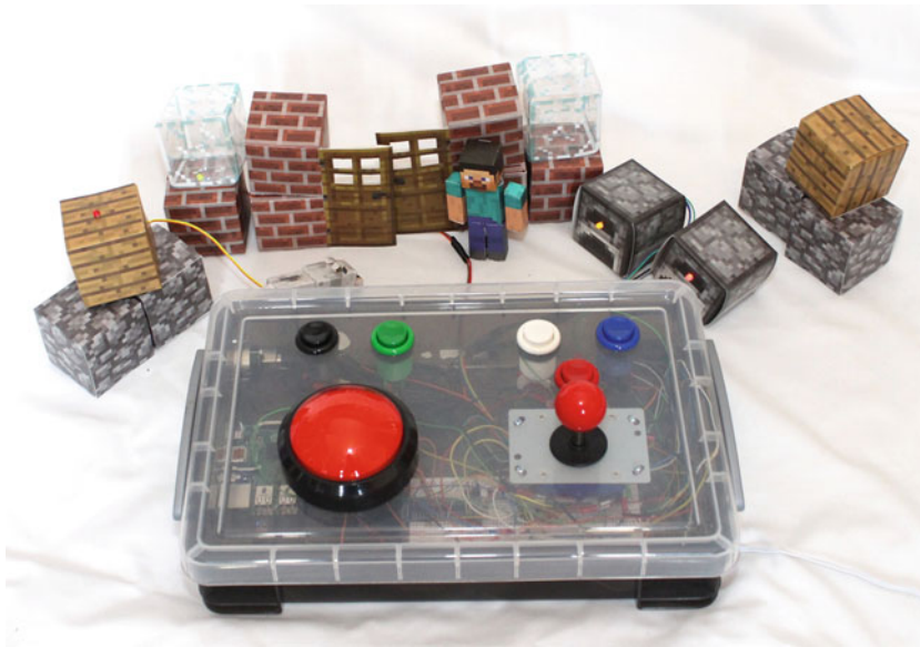
Figure 9-5. Minecraft blocks with tri-color status LEDs
