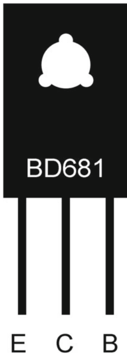
Figure 4-20. BD681 Darlington Transistor pinout
