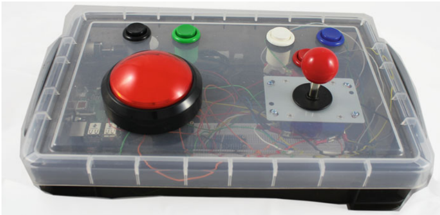
Figure 3-21. Enclosure with joystick for the arcade game
